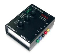
The COM01 tester will integrate with most standard alternator and regulator test bench equipment. The tester is a compact electronics device that allows controlling an automotive alternator output with BSS/LIN interface. The COM01 tester will act as the master communication device and the alternator will operate as the slave.
