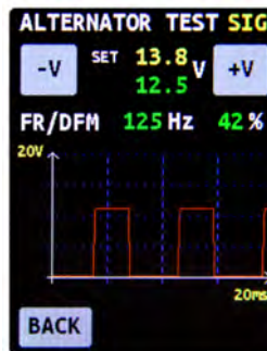
Fig. 8. Alternator diagnostic window when one of the following alternator types "SIG", "RLO", "RVC", "C KOR.", "P/D", "C JAP." is selected.
