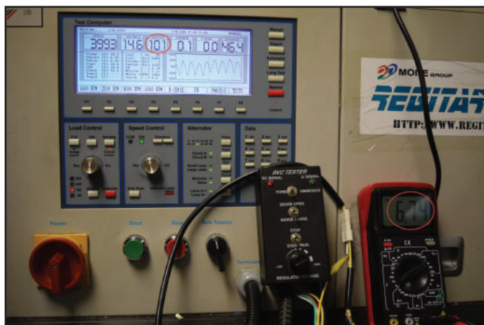
Figure 10 – Here is the readout on the Valeo/Hyundai alternator running at 4,000 RPM under a 100 amp load. Notice that the FR terminal voltage on the DVM has dropped as expected.
